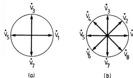
Fig. 2. Output voltages in multiphase rectifier
