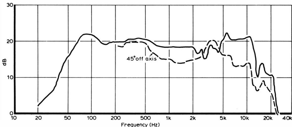
**Fig. 2.** An alternative presentation of speaker directivity to that in Fig 1. The frequency response is plotted for the speaker axis and for other angular distances from the axis.
