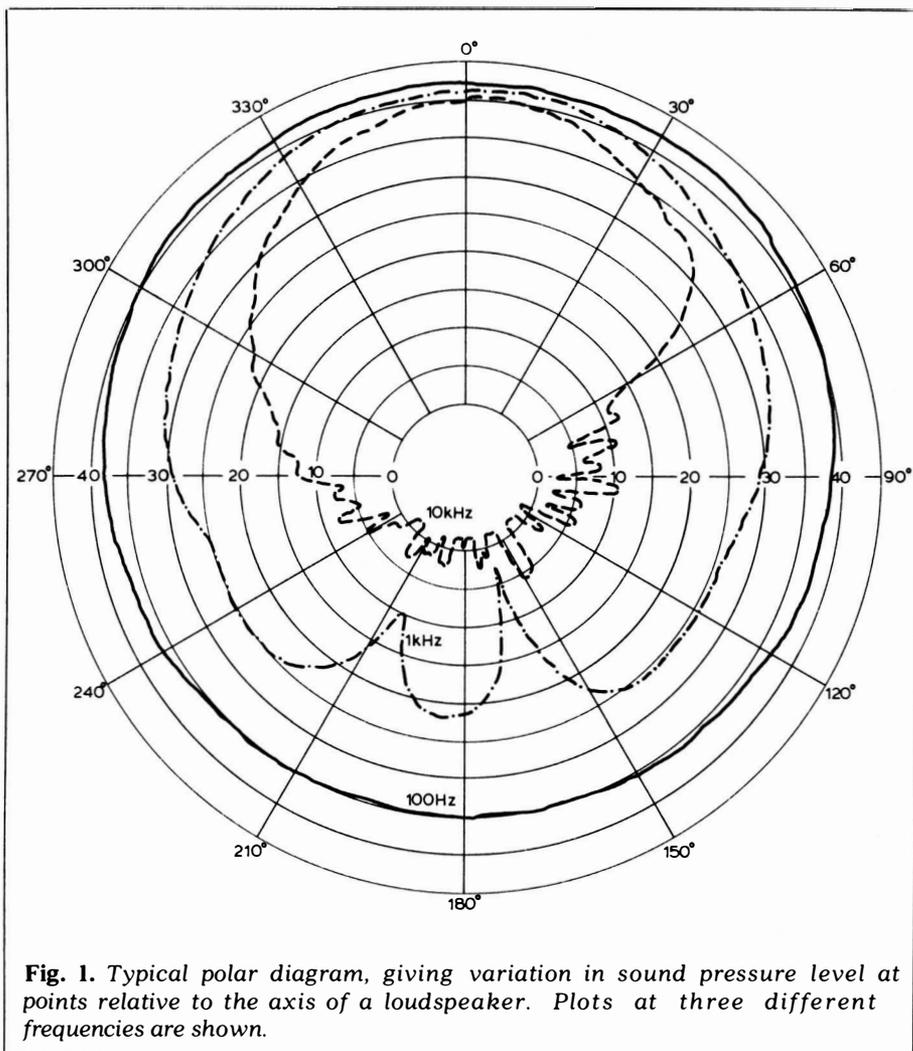
Fig. 1. Typical polar diagram, giving variation in sound pressure level at points relative to the axis of a loudspeaker. Plots at three different frequencies are shown.
