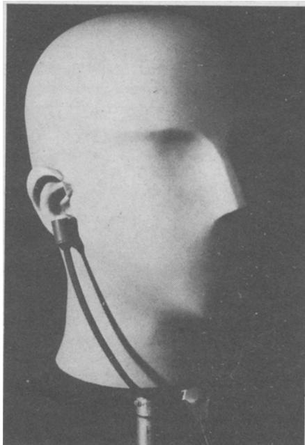
*Sennheiser microphone and artificial head assembly.*
