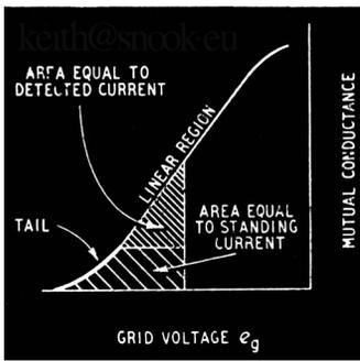
When the valve is to be used as a modulator, we shall apply a composite signal  $e_1 \sin \omega_1 t + e_2 \sin \omega_2 t$  to the grid, giving  $I_a = I_o + g_m(e_1 \sin \omega_1 t + e_2 \sin \omega_2 t) + B(e_1 \sin \omega_1 t + e_2 \sin \omega_2 t)^2 = I_o + g_m(e_1 \sin \omega_1 t + e_2 \sin \omega_2 t) + B(e_1^2 \sin^2 \omega_1 t + e_2^2 \sin^2 \omega_2 t + 2Be_1e_2 \sin \omega_1 t \sin \omega_2 t)$ .
