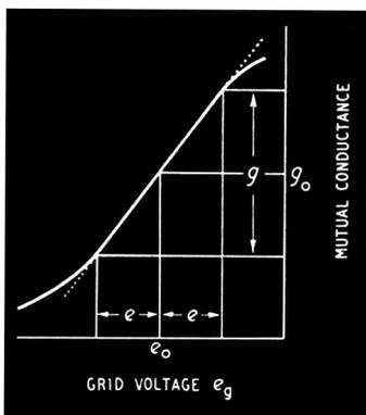
Fig. 1. The simplest type of valve  $g_m - e_g$  characteristic has a relatively long linear section.
