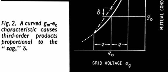
Fig. 2. A curved  $g_m - e_g$  characteristic causes third-order products proportional to the "sag,"  $\delta$ .
