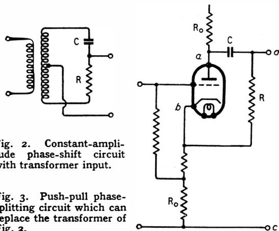
Fig. 2. Constant-amplitude phase-shift circuit with transformer input.
