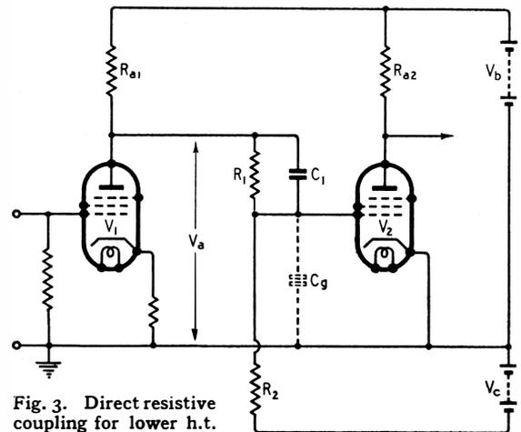
Fig. 3. Direct resistive coupling for lower h.t.
