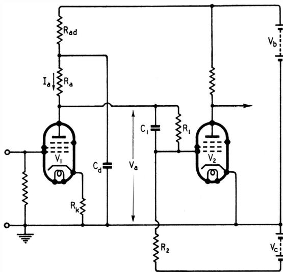
Fig. 5. A direct coupling used in wideband amplifiers.
