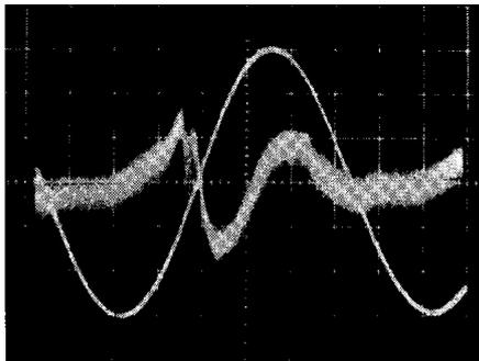
FIG.3 Distortion factor across R-jx load (8 Ω) with 70 dB (3162x) gain, 1 kHz 28 V RMS. Peak distortion = 0.016%
