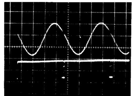
FIG. 9 Protection transistor switching at  $400\ \text{Hz}$  when driving load of  $Z=5.4\ \Omega$ ,  $\phi=48^\circ$  (voltage limiter on).
